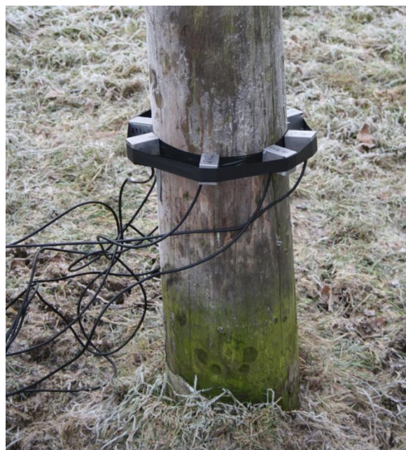
Figure 8 - Band of sensors fitted to pole
